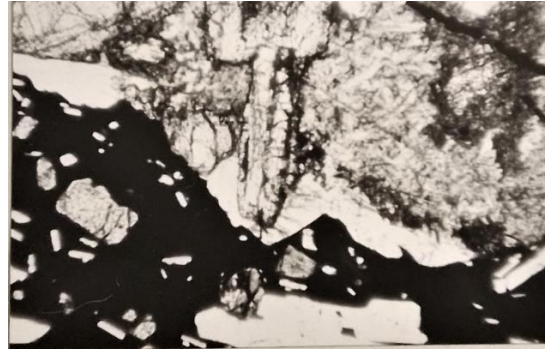
Contact of the highly altered first- and vitrophyric third-phase sills; the latter has idiomorphic phenocrysts of plagioclase and olivine, while the former is highly altered.
