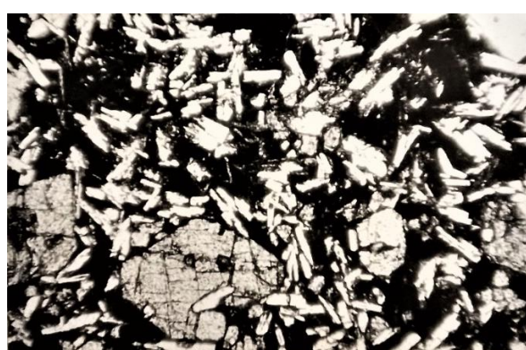
Away from glomeroporphyritic texture, idiomorphic plagioclase and olivine phenocrysts in fine-grained groundmass with seriate texture
