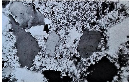
Z.472.5 corroded quartz grains separated by recrystallised matrix of quartz, feldspar, epidote, chlorite and calcite.
